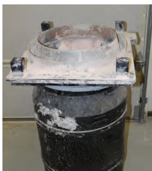
Slide Gate with Drum
