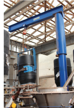
Jib Crane and Drum Handler
