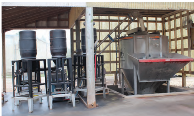
Closed System: Manual Drum Feeder to AMC with Hand Crank Dispensers
