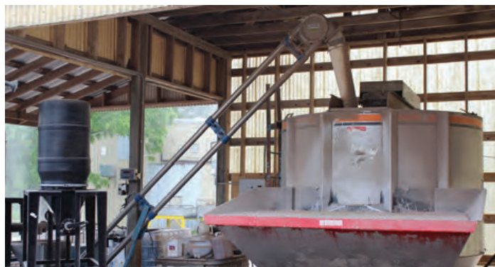
Closed System: Manual Drum Feeder to AMC
