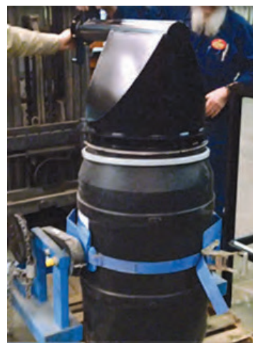
Feeder hopper and auger
