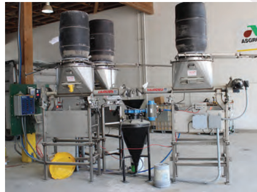
Automated Feeder Coupled to Autocharger (tied to plant automation)
