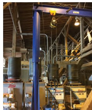
Ranco Powder Feeder with Jib Crane
