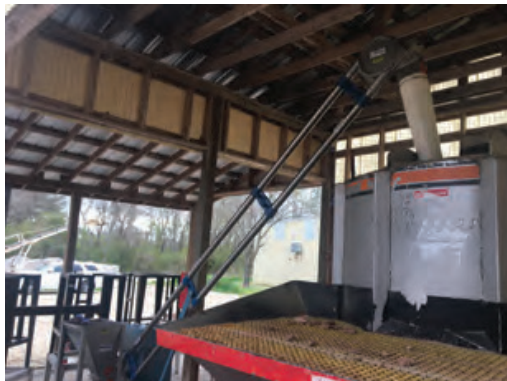
Aero Matic Conveyor (AMC) with Dust Collector
