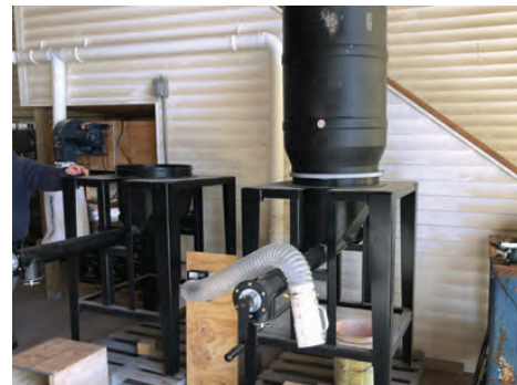
Manual Drum Feeder with Hand Crank
